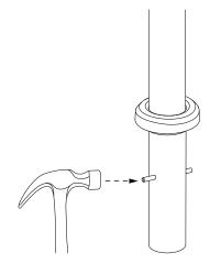
**NOTE:** In some cases the existing locking pin will need to be cut to a shorter length so it can fit into the new ground socket. Bolt-cutters are recommended if this is required. For any queries, please contact the Hills Customer Service Centre: Australia - 1300 327 293 / New Zealand - 0800 021 027.
